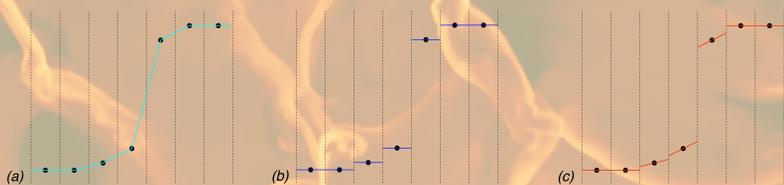
Panel (a) shows a discrete source function (black dots) which is continuously connected by linear interpolants as done with the DELO method. In panel (b) the source function is (conservatively) reconstructed by a piecewise constant function. Panel (c) shows a piecewise linear reconstruction using the minmod slope limiter. The piecewise continuous reconstructions allow for true discontinuities at grid interfaces.
